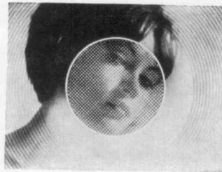
Microprism screen is fuzzy = unsharp
